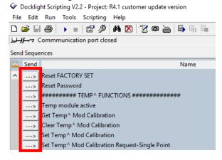
With Docklight you can calibrate the conductivity probe, set emails and phone numbers for alarms and others. To execute the command, click the arrow, located to the left of each command.
