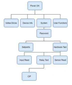
Through the main controls go to RELAY TEST and open the CIP Pump (CIP) by pressing ENTER. The CIP solution will start flowing through the CIP line. Once the solution reaches the beaker, stop the CIP pump by pressing ESC. Reconnect the check valve. The CIP line is now primed.
