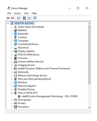
Open device manager and click the PORTS tab. Check the virtual port assigned to the connected USB.
