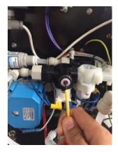
Replace these flow restrictors with the desired ones. First remove the old flow restrictor from the flow restrictor housing by gently pushing with a screwdriver. Then insert the desired flow restrictor by reversing the procedure described above.
