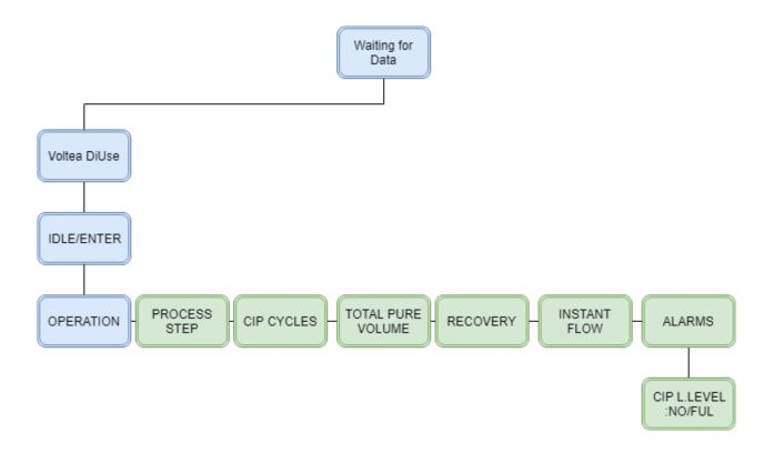
**NOTE:** CIP solution level is calculated based on the CIP's pump capacity to exhaust the 1L of CIP solution. For this reason, it is mandatory to reset the CIP alarm once the CIP bottle is refilled. Around 36 ml of CIP solution is used per CIP event.
