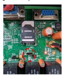
Connect the laptop to the system using a USB 2.0 cable (micro-USB to USB) placed directly into the micro-USB port of the PCB.
