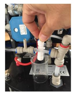
Use a small beaker to collect the acid during priming.
