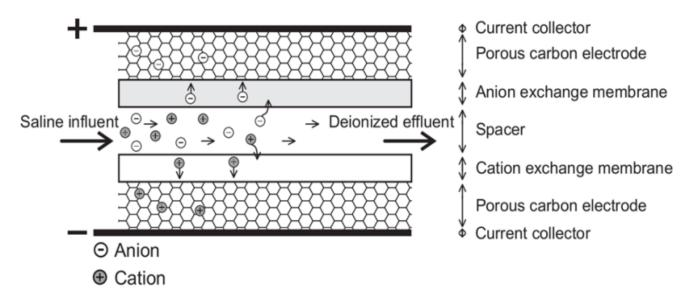
A CapDI module consists of a housing which contains multiple stacks of parallel unit cells. Each unit cell consists of two porous carbon electrodes separated from each other by a spacer. On top of the electrodes,
