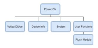
Flushing the module is required for at least 15 minutes before starting operation for the first time. To flush the module, select the built-in function via the LCD screen.
