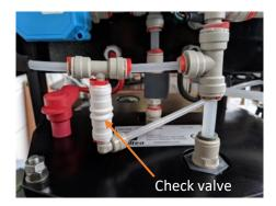
• Disconnect the CIP line check valve.
