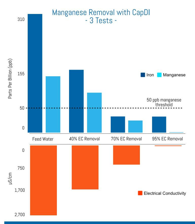
CapDI was tested to evaluate its efficacy as a chemical-free way to remove manganese below the regulatory requirement level of 50 ppb. The results were a smashing success! Testing that was performed included 3 conditions: 40, 70, and 95% electric conductivity (EC) removal, with the manganese removal as noted.
