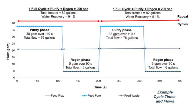
In the above flow diagram example, it is shown that the peak flow is 38 gpm and the net pure flow rate is 22.8 gpm. The net pure is lower than peak as it is averaged over the total cycle time, accounting for time when the system is in regeneration and not producing purified water.
