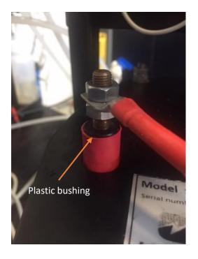
• Each module has one red and one black electrical terminal, with each terminal having two M8 nuts. Unscrew one of the nuts from the red terminal. Place the red cable from the system on the red electrical terminal, then screw the nut back on. Tighten using two size 13 wrenches, one on the top nut and one on bottom nut. Repeat the process with the black terminal and black cable. Be sure the bottom nut isn't sitting on the plastic bushing.
