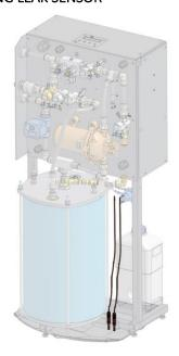
• Take the two sensors and place them in the clamps as shown in the image. The tip of the sensor should be in contact with the leak tray.
