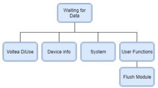
Flushing the module is required for at least 15-20 minutes before starting operation for the first time. To flush the module, select the built in function via the LCD screen.
