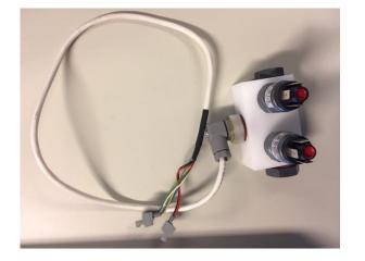
Disconnect the external EC probe from the PCB and connect the EC probe mounted on the special manifold. Fill the manifold with the calibration solution. Voltea suggests using a 147μS/cm standard solution.
