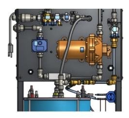
• DiEntry is equipped with a system pump to maintain the operational flow.
