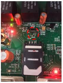
Connect the laptop to the system using a USB 2.0 cable (micro-USB to USB) place directly into the micro-USB port of the PCB.
