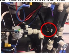
The system comes with a GSM communication antenna. To utilize this feature, insert a dataready, unlocked SIM card into the SIM slot. System needs 2G coverage to communicate.
