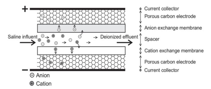
A CapDI module consists of a housing which contains multiple stacks of parallel unit cells. Each unit cell consists of two porous carbon electrodes separated from each other by a spacer. On top of the electrodes, ion exchange membranes are placed. The spacer between the membranes acts as a flow channel to transport the water to be desalinated.
