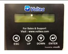
The system can be controlled using the LCD screen and the keypad. Navigate through the screens using the **UP** and **DOWN** buttons, confirm selection with **ENTER**, and return to the previous screen by pressing **ESC**.
