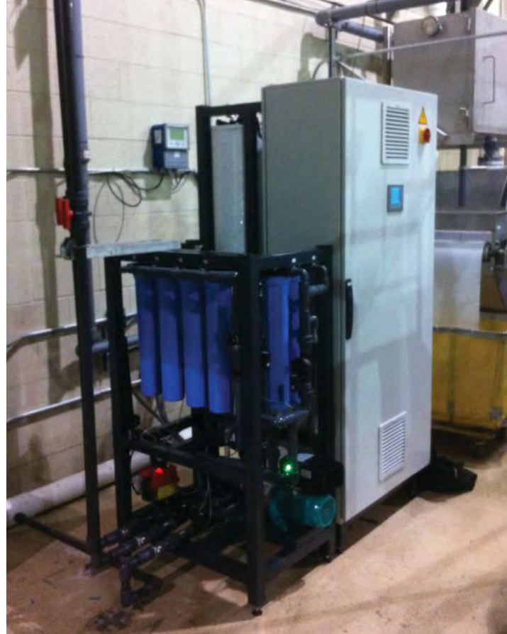
This membrane capacitive deionization technology uses electro-desalination in a two-step process.
